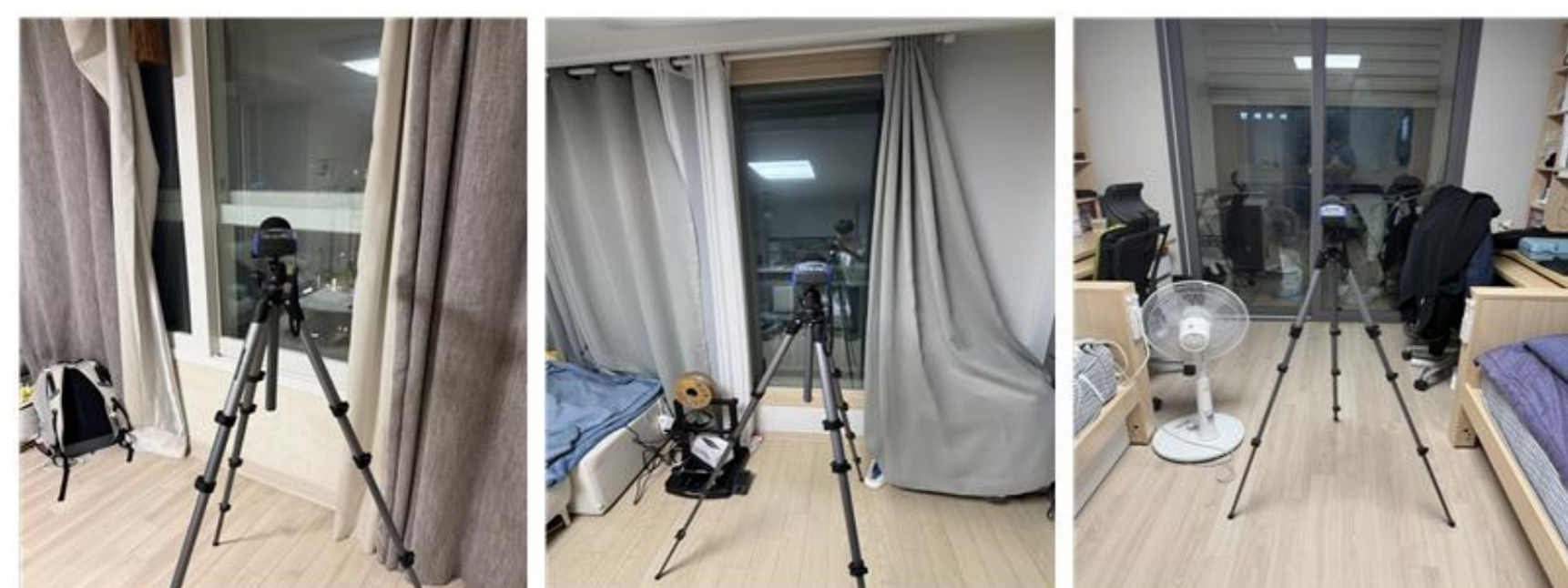
Fig. 4 Indoor Noise Measurements
